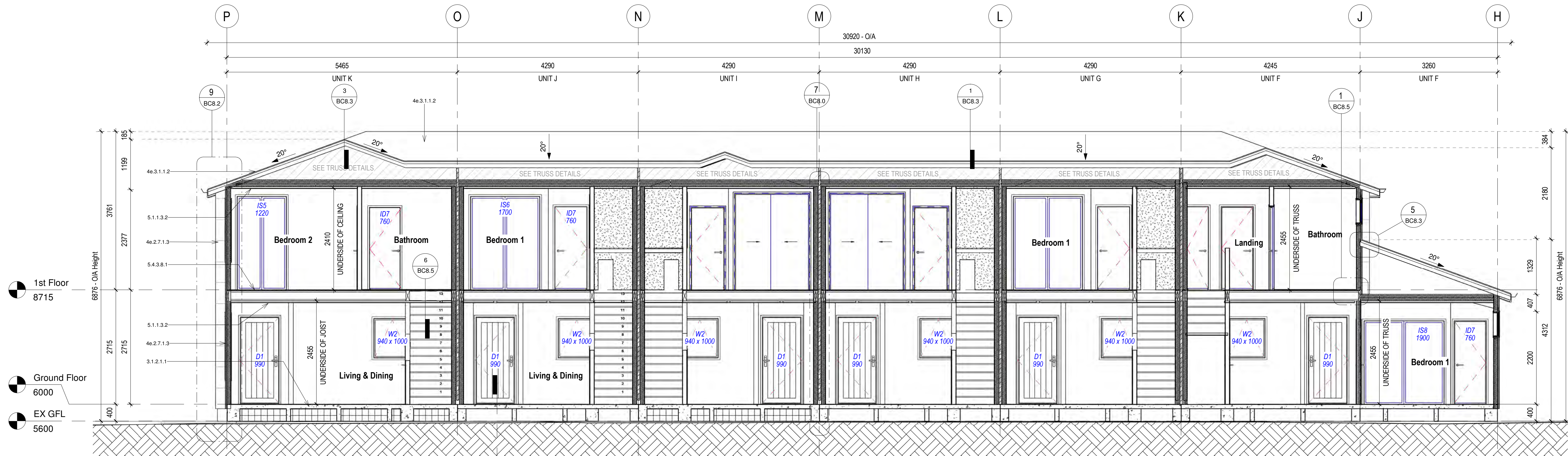
A SECTION 'A' - BLOCK 3 1 : 50
